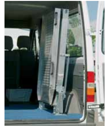
The RRD-ramp is rotatable inside and outside.
